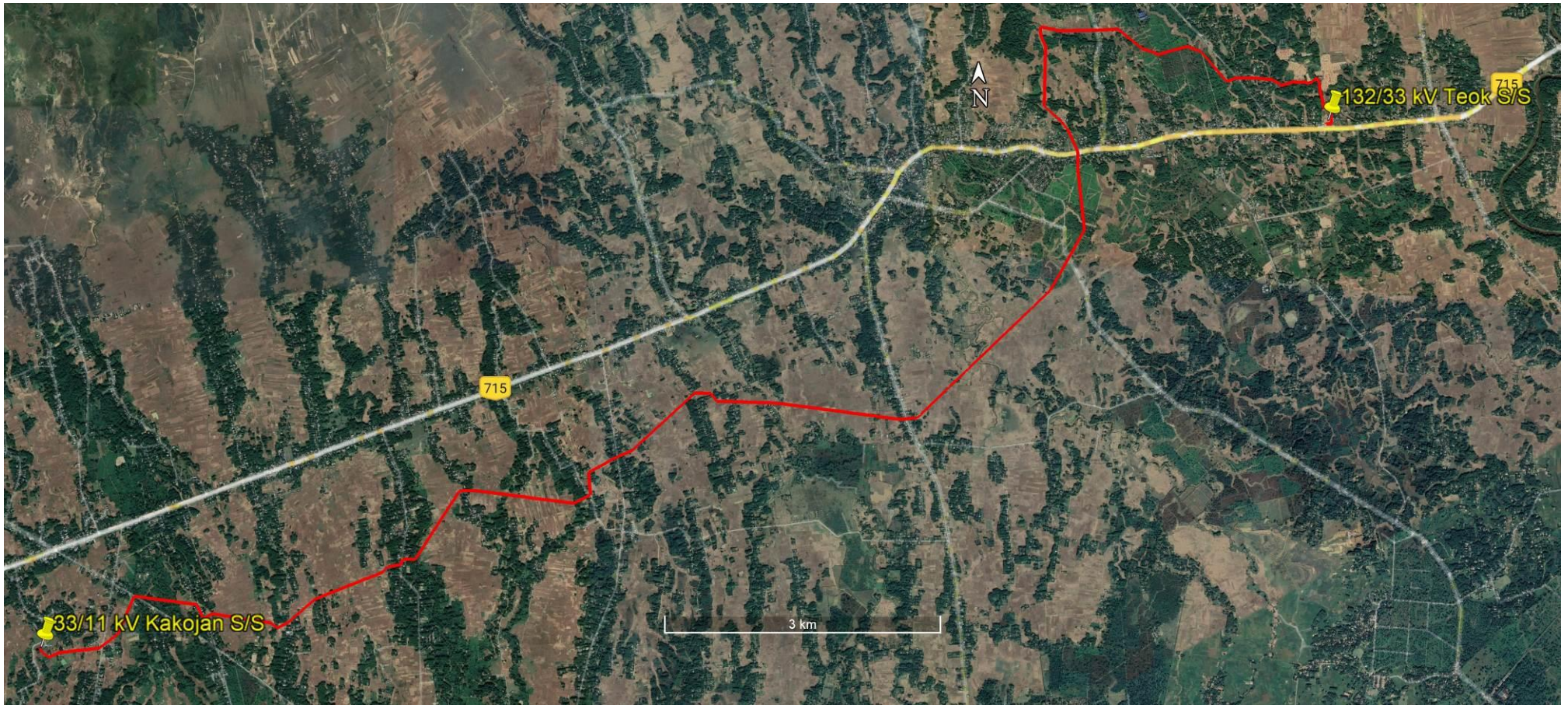
Figure 4.6: Satellite Imagery Showing Route of 33 kV line from 132/33 kV Teok (new) S/S to 33/11 kV Kakojan (existing) S/S
