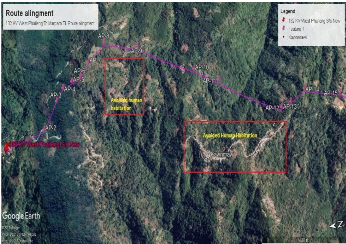
Avoidance of habitation area (AP-1 to AP-16) for West Phaileng- Marpara 132kV line in Mizoram
