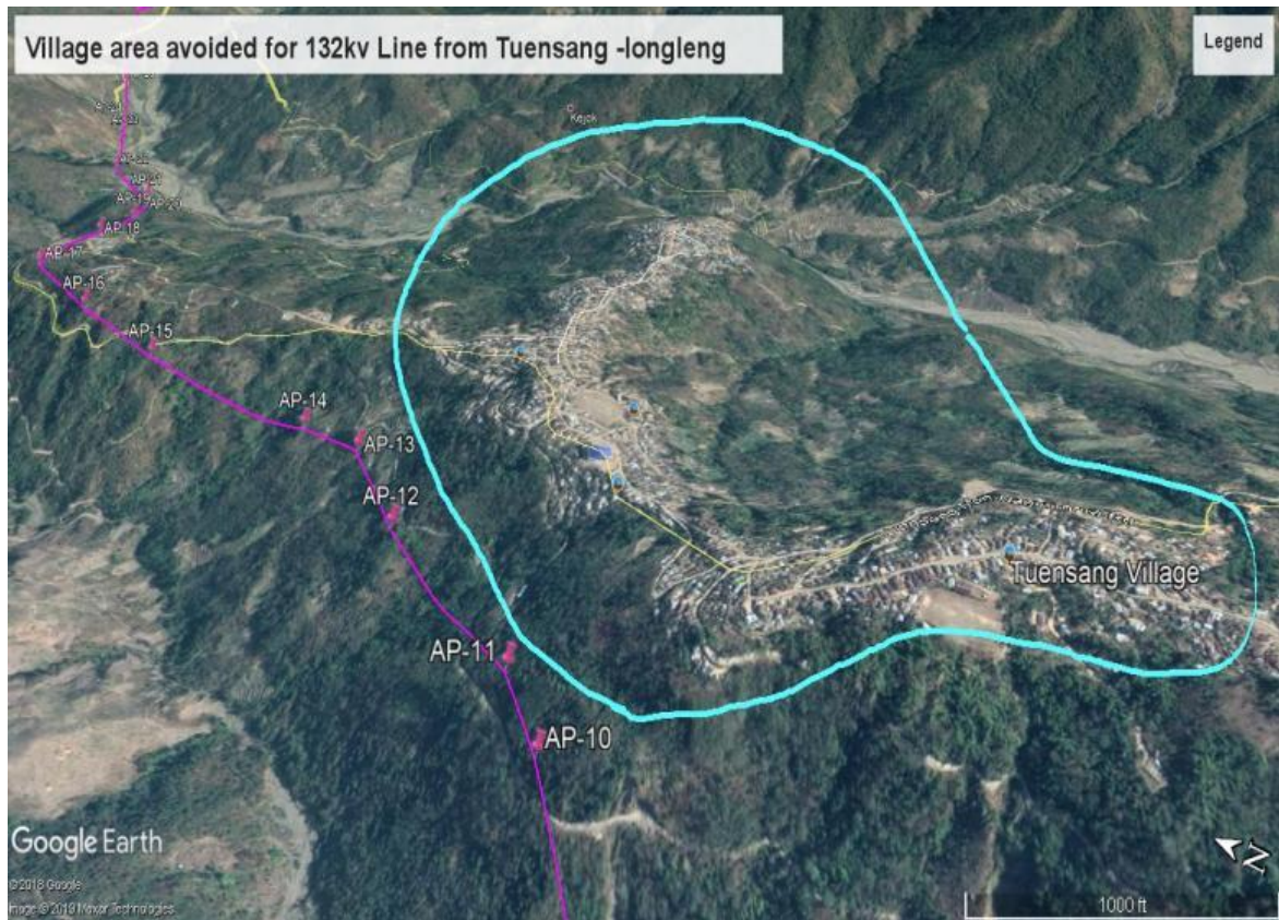
Avoidance of habitation area for Tuensang – Longleng Complex 132kV line in Nagaland
