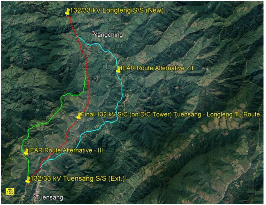
Figure 4.1: Satellite Imagery Showing Route of 132kV S/C (on D/C Tower) Tuensang – Longleng Line
